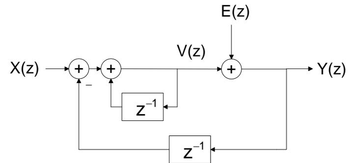
2<sup>nd</sup> order  $\Delta\Sigma$  modulator with one bit quantization
